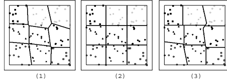
Fig. 9. Constructed boundary in a 9-class problem: (1) Linear (91.2%), (2) Ideal decision tree (97.8%), and (3) The proposed method (93.5%)
