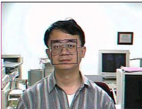
Fig. 3. One example of the approximate face-only image delimited by a black-line rectangle which is extracted based on the two eyes marked in white circles
