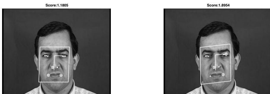
Fig. 6. Typical detection result. The best face hypothesis (left) and the worst-score face hypothesis below a distance threshold (right). Features that formed the triplets are marked. The worst face hypothesis has a quite high shear, and consequently high score because high shears were unlikely transformation in the training set
