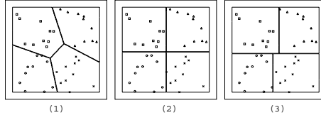
Fig. 8. Constructed boundary in a 4-class problem: (1) Linear (90.4%), (2) Ideal decision tree (97.5%), and (3) The proposed method (92.8%)
