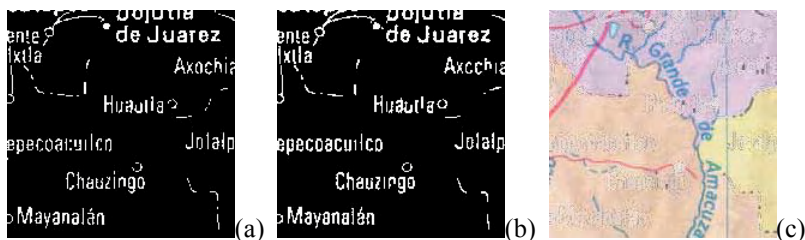
Fig. 5. (a) Binary sub-image after thresholding the image resulting when adding pixel-to-pixel the 24 sub-images shown in Fig. 4. (b) Resulting image after filling the gaps on (a). (c) Resulting image after eliminating the pixels on Fig. 1 as explained in the text.
